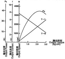
Operating Voltage = 12VDC Rated Output Power = 25 Watts Rated Current = 3.5 Amps No load Speed = 3000 RPM Standard Protection = IP35 Configuration = Enclosed PM Brushed Minimum Brush Life = 2000+ Hours Weight = 1 Kilogram
